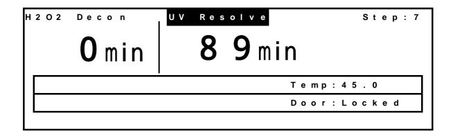
**10.** After  $H_2O_2$  gas resolution,  $H_2O_2$  decontamination has been completed. The following display will appear. Open the outer door and disconnect the cable of  $H_2O_2$  Generator from the connector in the chamber. Then take out the  $H_2O_2$  Generator.
